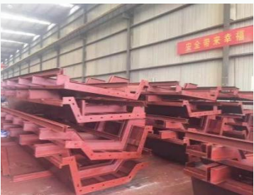
Overpass tie beam formwork
