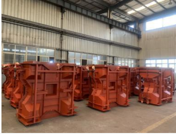
Four corner hollow block formwork
