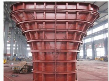
High-way pier column formwork
